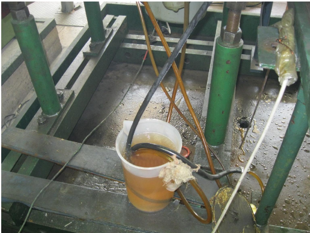
Photo No.3 – the color of fuel after test
